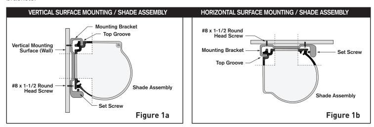
**Step 1.** Determine the desired location for the mounting brackets, making sure that they are plumb and level. Using a pencil, mark the 2 hole locations in the bracket. Using a 1/8" bit, drill holes approximately 1-1/2" deep at both hole locations. Repeat for the mounting bracket on the other side, and the center mounting location on 10' to 12' models.
